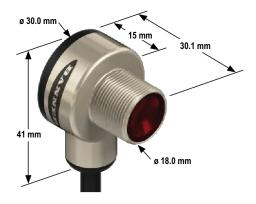
Opposed, Polar Retroreflective, Diffuse and Fixed-Field Models Suffix E, R, LP, DV and FF
