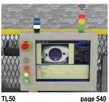
Banner's E-Stop Button and Signal Tower Lights with audible alarms provide highly visible and audible fault detection. The E-Stop button is setup for use in case of an emergency as a part of safety control.
