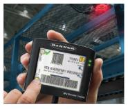
RD35 Handheld Remote Display Used for- programming
