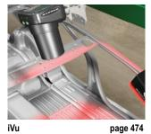
Banner's iVu Image Sensor with C-Mount Lens inspects a car frame to ensure it has been correctly assembled.
