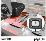
After the frozen dinner is placed in the carton, Banner's iVu BCR reads a 2D code on the carton to ensure it is the correct carton to prevent packaging errors.
