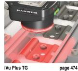
To verify the expected number of holes exists on a small metal part, the iVu Plus TG Image Sensor with Multipoint Inspections can be configured for multiple regions of interest (ROIs) to ensure holes exist and were punched in the correct place.
