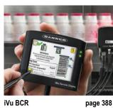
The iVu Bar Code Reader (BCR) with a remote touch screen display simplifies barcode reading of various symbologies including 1D, 2D Datamatrix, and PharmaCode. Inspection configuration can be setup easily using the touch screen without the need of a PC
